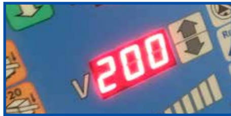
IT_ Controllo peso film. EN_ Film weight check. FR_ Calcul poids de film. DE_ Kontrolle Foliengewicht. ES_ Control peso film.
